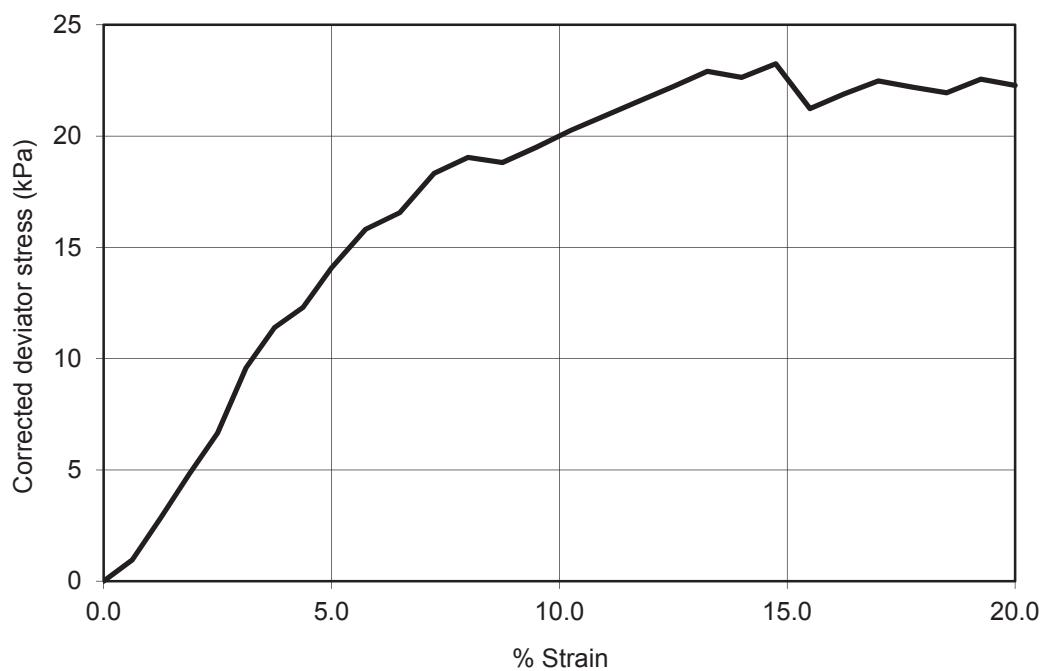
Strain at failure % 14.8 Cohesion C<sub>u</sub> (kPa) 12
