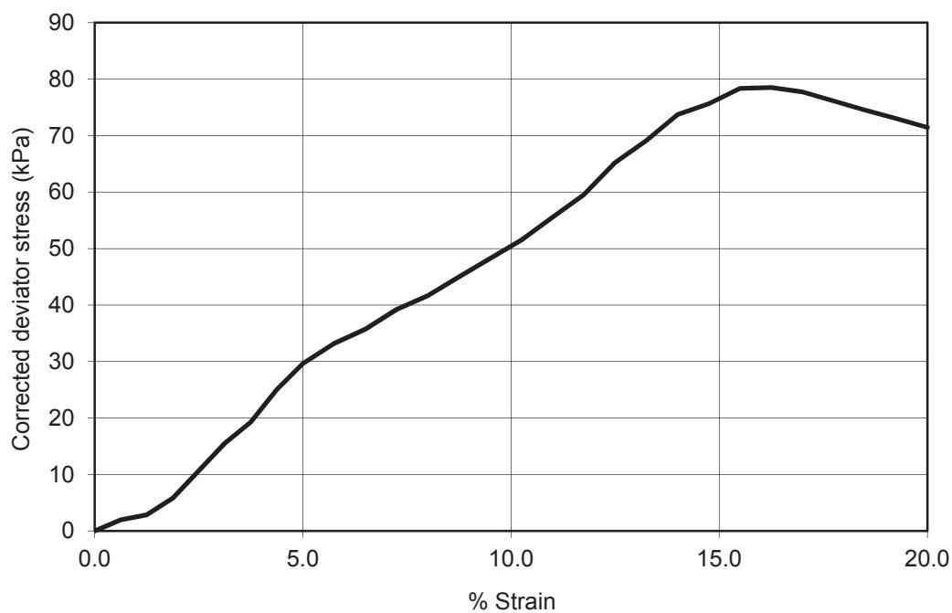
Strain at failure % 16.3 Cohesion C<sub>u</sub> (kPa) 39
