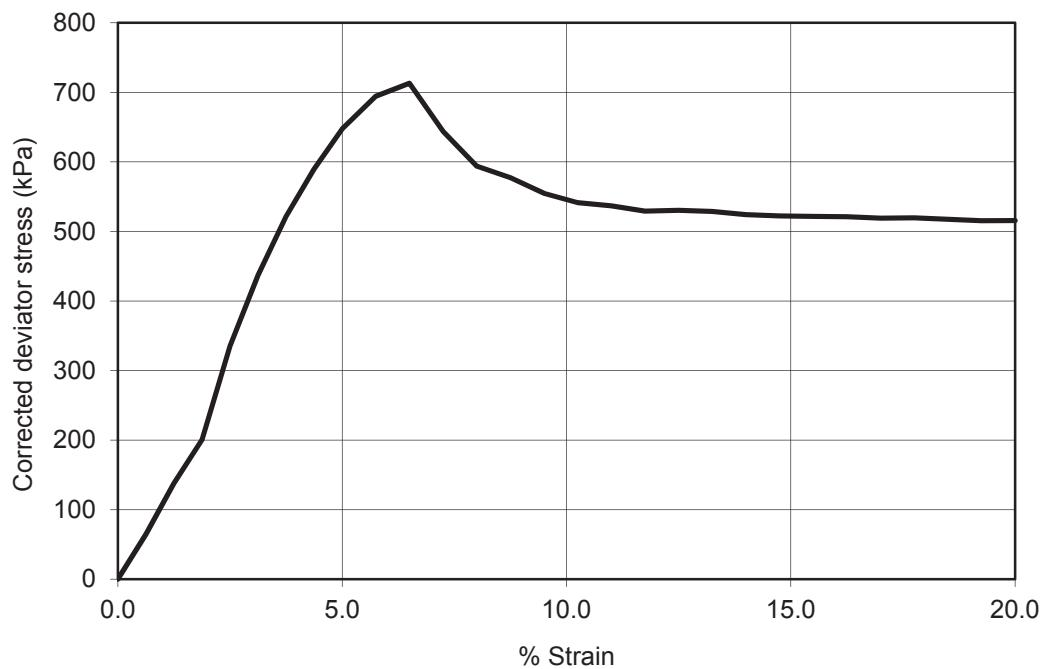
Strain at failure % 6.5 Cohesion C<sub>u</sub> (kPa) 357
