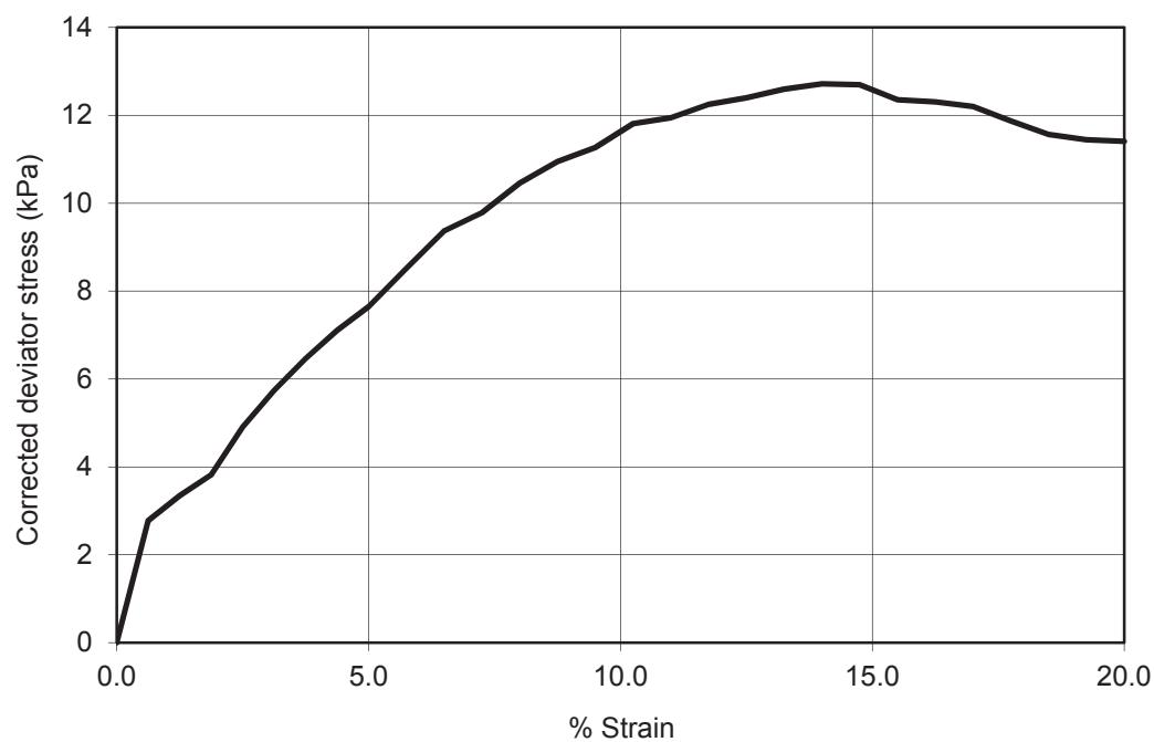
Strain at failure % 14 Cohesion C<sub>u</sub> (kPa) 6
